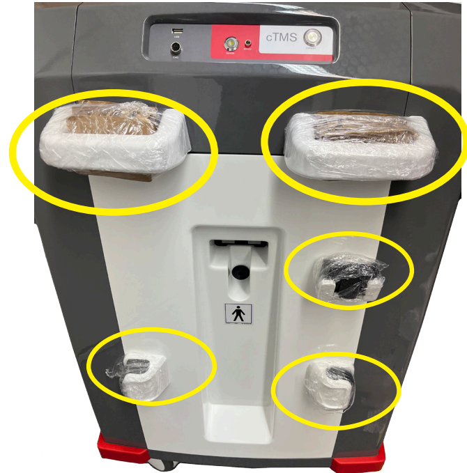
Fig. 2-3: Main chassis with handle protectors (yellow circles)
