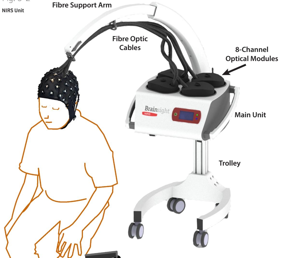
scanners) and either switch the fibres connected to the block, or purchase an optical module along with the fibres to simplify switching back and forth. The unit is held on a mobile trolley that includes an articulated arm to hold the fibres.
