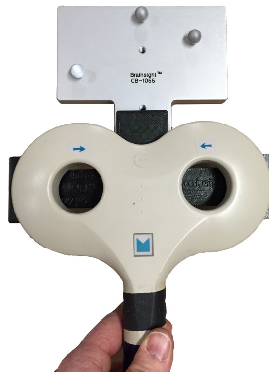
B: Coil placed in the jig for calibration.
