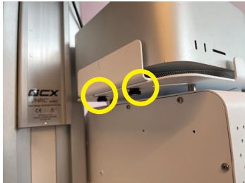
B: Computer Tray Side Bar w. thumbscrews
